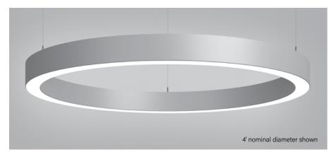
High Performance 2" Aperture Circle (HP-2 C) is a patented, circular LED luminaire. Constructed with an extruded aluminum body and single-piece direct diff ser, the HP-2 C provides a seamless finish aesthetic. Delivering excellent performance using an advanced optical design and mid-power LEDs to achieve 90% of initial light output at 100,000+ hours.
