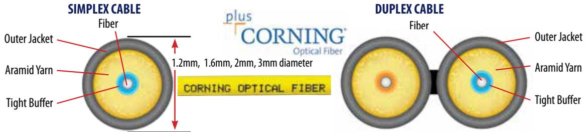
Corning's new SMF-28® Ultra optical fiber is the first in the market to combine the benefit of industry-leading attenuation and improved macrobend performance in one fiber. This premium single-mode fiber is designed for long-haul, metro, access, and fiber-to-the-home (FTTH) applications, and is fully backward compatible with the installed base of legacy single-mode fibers.
