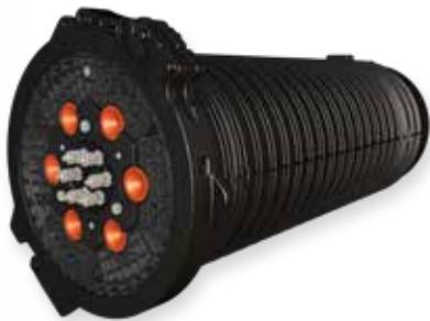
**APEX-2S:** Dimensions: 20" x 12", Weight 22lbs(no trays), Splice Capacity 216 Single/432 Mass, Tray Capacity is 6, Single Port Cable OD 10-28mm, Multi-Drop Port Cable OD 5-9.9mm.
