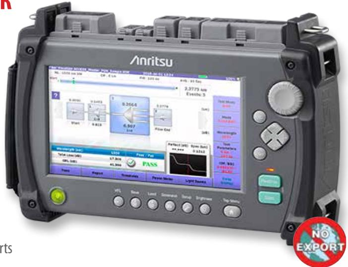
The ACCESS Master MT9085x is a handheld complete Fiber Optic Cable tester for performing all optical pulse tests, optical loss/power measurements and optical fiber end-face inspections. Ideal for FTTx, PON, Metro WDM. The MT9085 now features an 8-inch TFT 16:9 wide touch screen display for use indoors and outdoors while providing a rotary knob and new short-cut function keys that simplify and minimize operations and time to complete a test.
