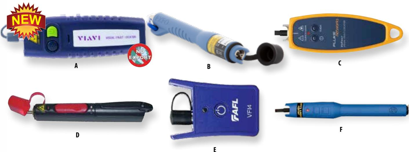
Fault Locators are a special class of light sources that emit a high intensity visible Red Laser into a patch cable or cable. This light can be used to both check the continuity of a fiber and identify the fiber's far end, or it can be used to visually identify the location of a fiber break. Most Fault Locators come optimized for singlemode fiber use; however they work equally as well with multimode fiber.
