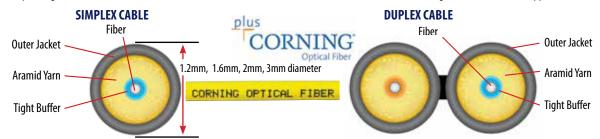
Corning's new SMF-28® Ultra optical fiber is the first in the market to combine the benefit of industry-leading attenuation and improved macrobend performance in one fiber. This premium single-mode fiber is designed for long-haul, metro, access, and fiber-to-the-home (FTTH) applications, and is fully backward compatible with the installed base of legacy single-mode fibers.
