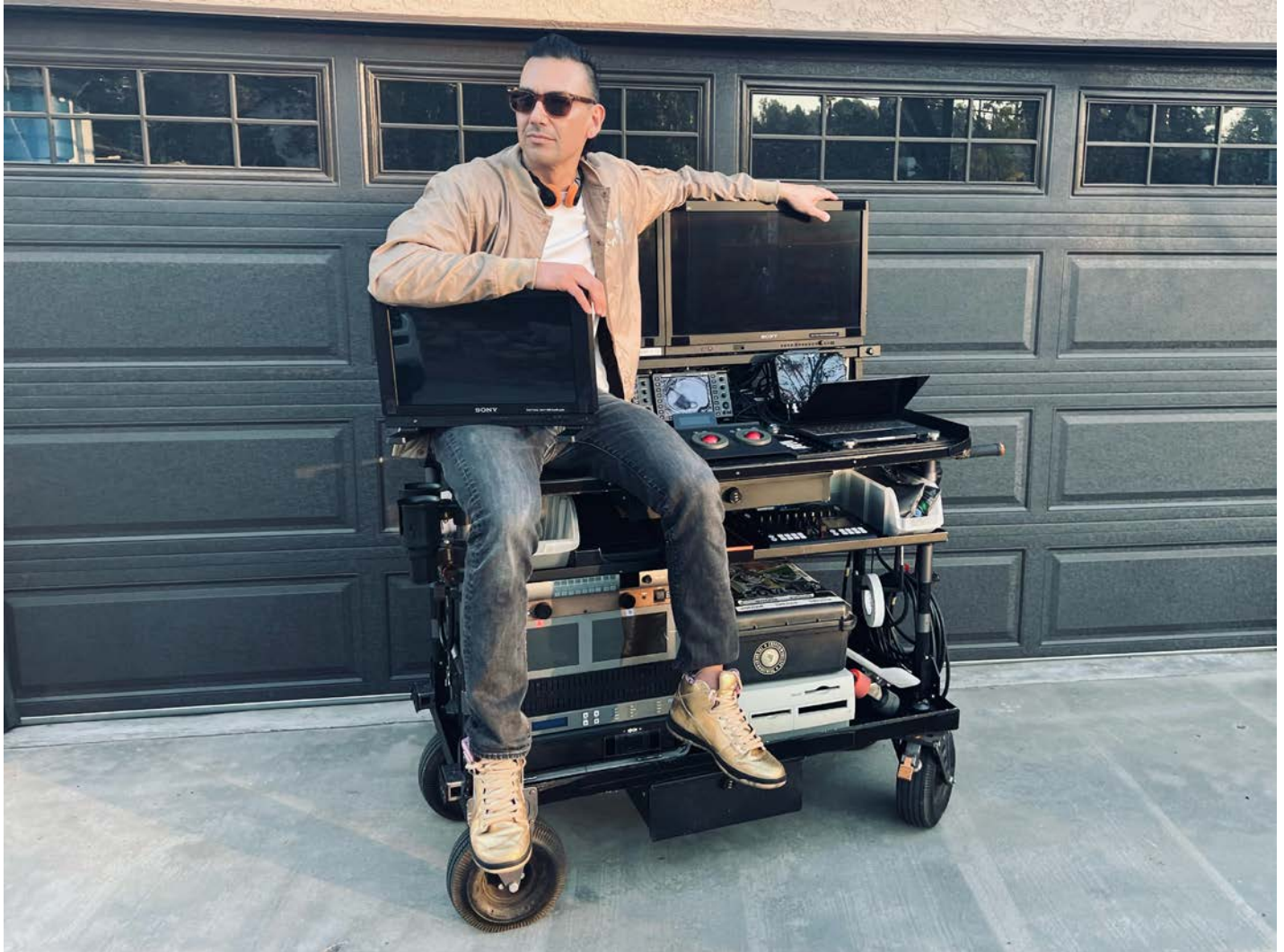
Tim Nagasawa sitting on his Inovativ Echo 48 DIT cart with a Sony PVM-A170, two Sony PVM-A250 monitors, two Leader LV5333, Odyssey 7Q+, AJA Frame Synchronizer, Four Teradek COLR, Blackmagic Smartvideo Hub 20X20, Tangent Element Color Correction Panel, 13" Macbook Pro, Decimator Quad Splitter, two Blackmagic UltraStudio HD Minis, backup RAID array housed in a vintage Apple, and skateboard.
