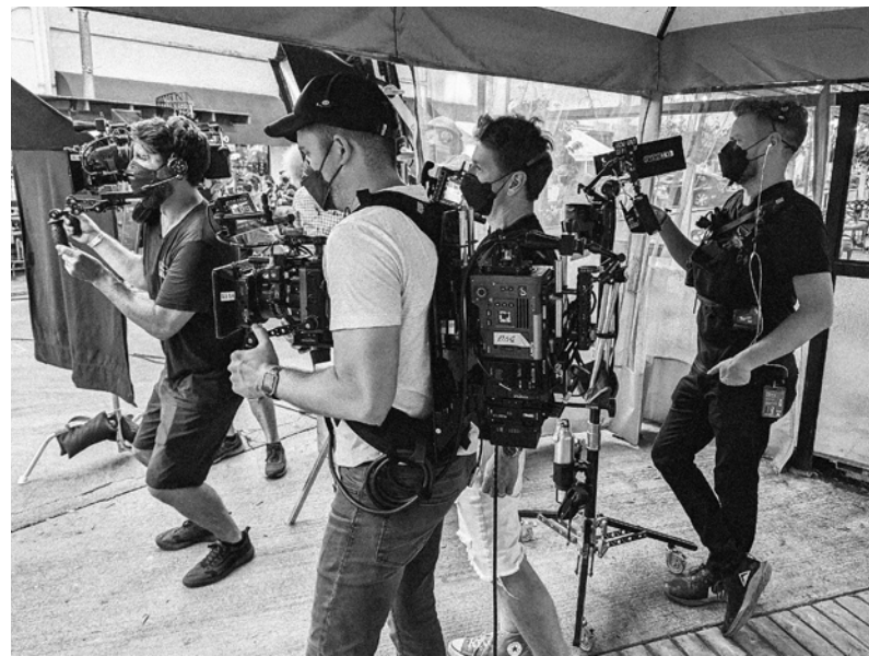
VENICE 1 in Rialto mode in foreground; VENICE 2 handheld in background. 1st AC Ben Steen at right.
