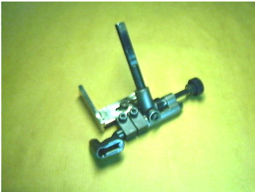
FCS 00011 Special guide for piping
