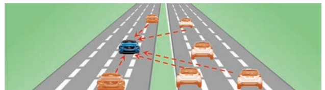
FIGURE 5. Network interference on a six-lane highway. Interference from interfering radars is aggregated and depends on the properties of the individual radars as well as on the placement of vehicles on the road.
