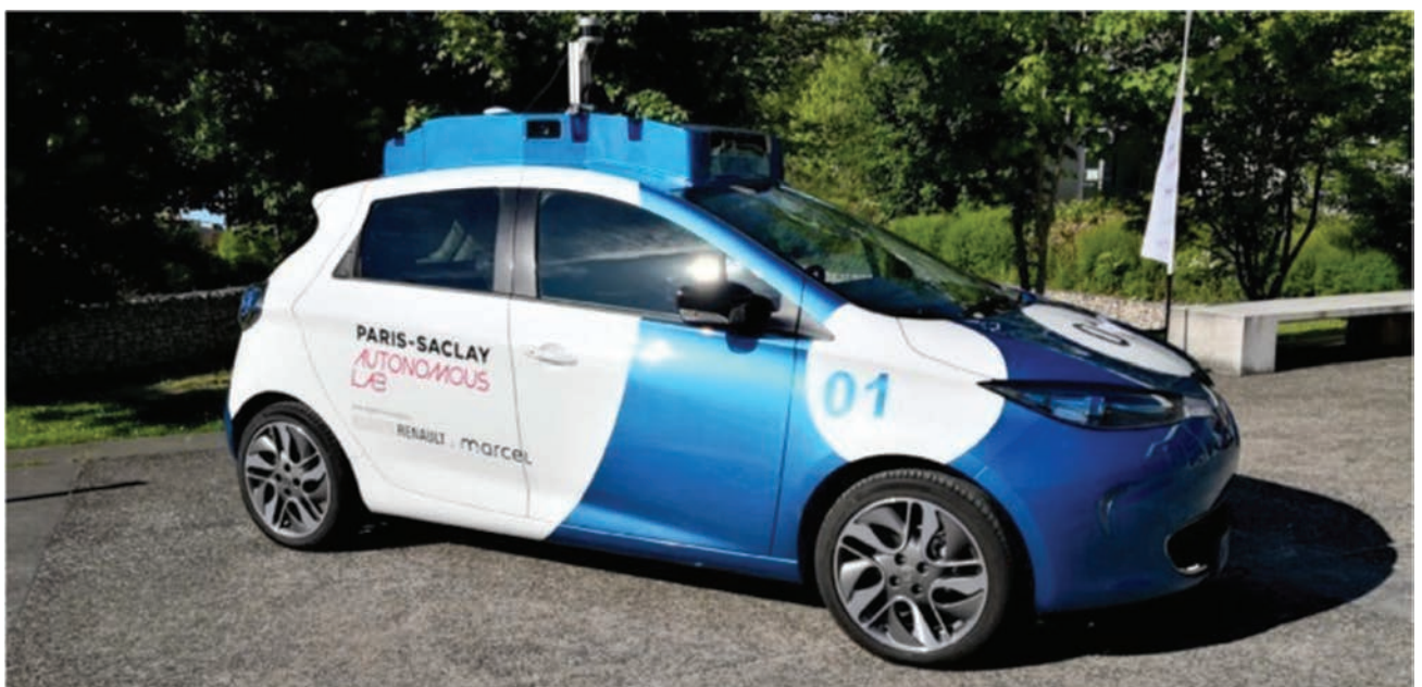
FIGURE 1. The autonomous vehicle prototype developed by Groupe RENAULT for the EVAPS project. The most evident sensor is the Velodyne UltraPuck lidar on top.
