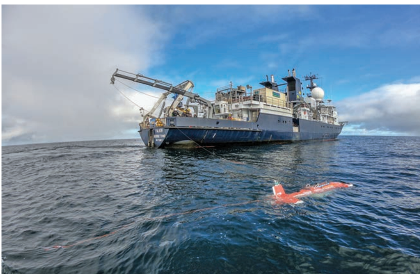
FIGURE 2. The exploration vessel Falkor launches a probe designed to acquire images from the seabed for a research project aiming to show how combining autonomous robotics and AI technologies can dramatically accelerate the exploration and study of hard-to-reach deep-sea ecosystems. (Source: Schmidt Ocean Institute.)
