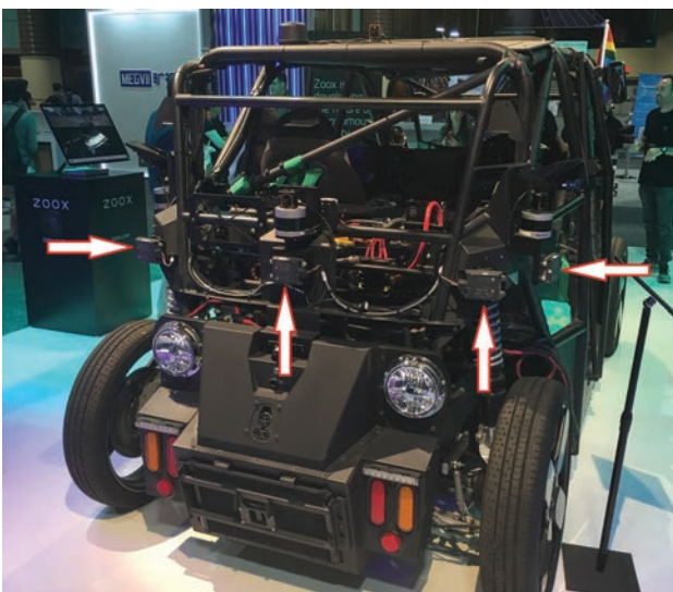
FIGURE 1. A Zoox autonomous driving vehicle, exhibited at the 2019 Conference on Computer Vision and Pattern Recognition, is equipped with 10 millimeter-wave (mm-wave) automotive radar sensors (marked by white arrows) at the front, rear, left, and right sides.
