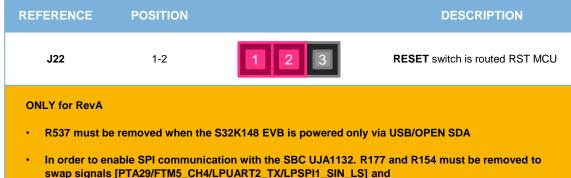
[PTA27/FTM5\_CH2/LPSPI1\_SOUT/LPUART0\_TX\_LS] by external wires.
