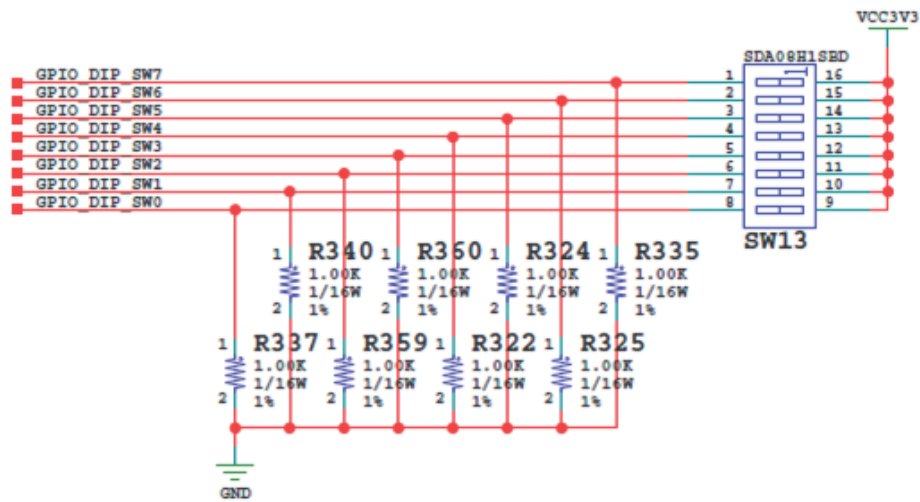
Figure 3-33: GPIO 8-Pole DIP Switch
