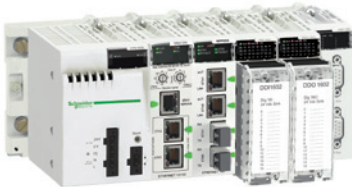
Modicon X80 EIO drop with CRA bus terminal module
