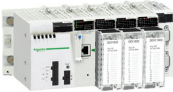
Ethernet Modbus/TCP DIO drop with PRA module
