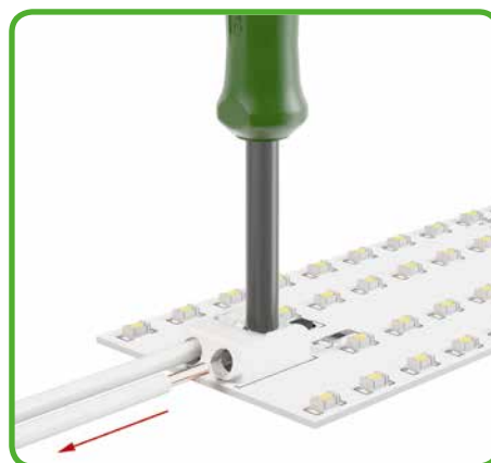
Inserting/removing fine-stranded conductors by lightly pressing on push-button (e.g., using a 206-861 operating tool).
