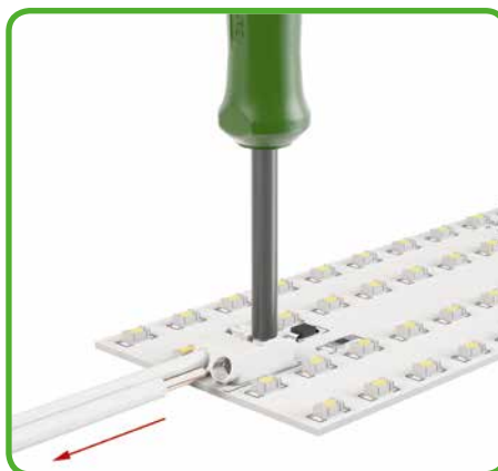
Inserting/removing fine-stranded conductors by lightly pressing on push-button (e.g., using a 206-860 operating tool).
