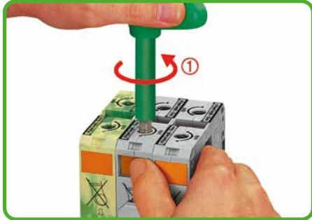
Rotate Allen wrench counterclockwise to the stop ①. Then, push in orange locking tab for hands-free wiring.
