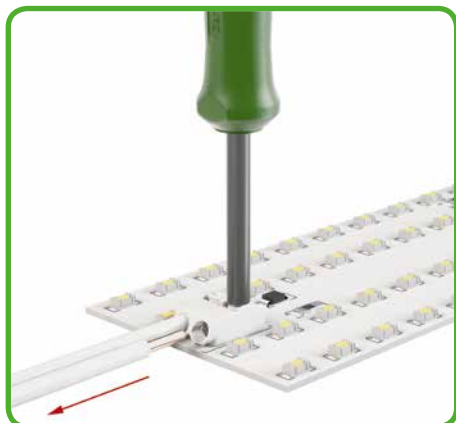
Inserting/removing fine-stranded conductors by lightly pressing on push-button.
