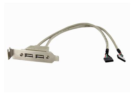
This 2 Port USB A Female Low Profile Slot Plate converts the USB pins from most AT style Pentium (and newer) motherboards to 2 standard USB A style ports. The plate can be mounted on the rear panel of a computer case, adding two USB A female ports for simple connection to USB peripheral devices.
