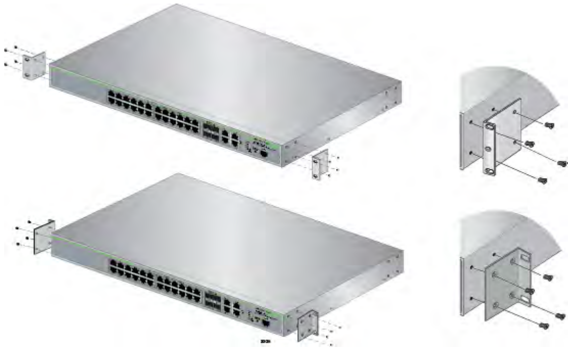
Figure 14. Attaching Brackets for Rack Mounting
