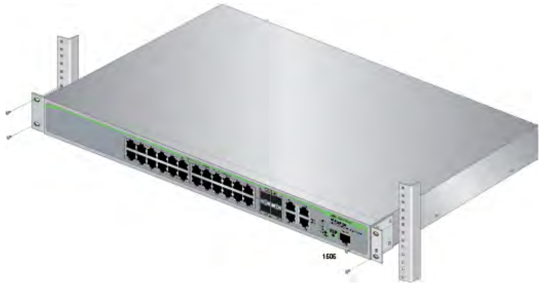
Figure 16. Mounting the Switch in a Rack
