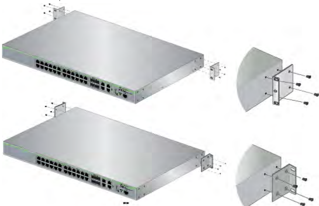
Figure 15. Attaching Brackets for Rack Mounting (Continued)
