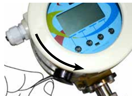
Fig. 39 Activation of the MC608B/R
