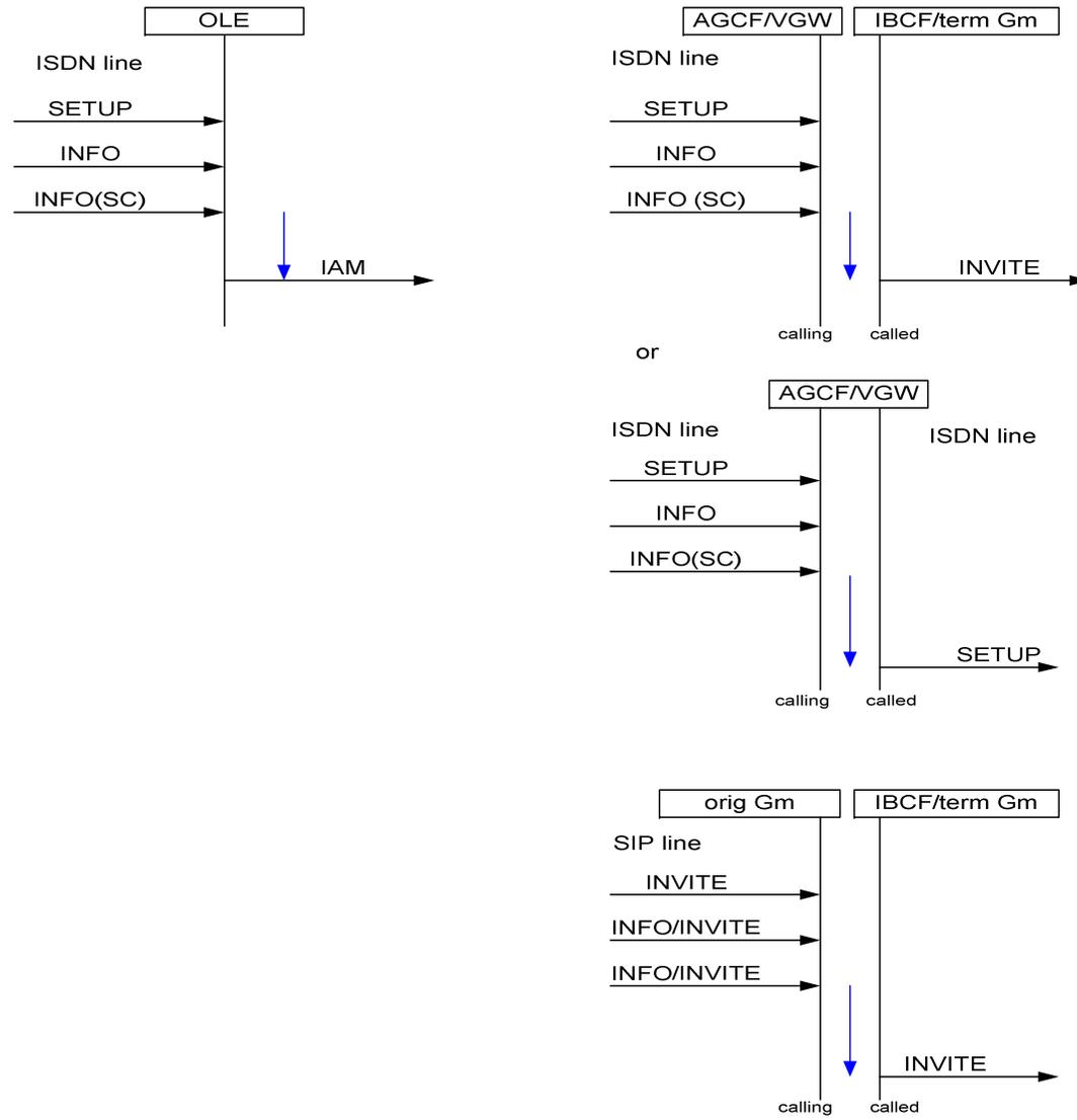
Figure 8: Call set up delay: Overlap sending is used
