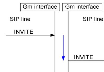
Figure 9: Call set up delay: en-block sending is used
