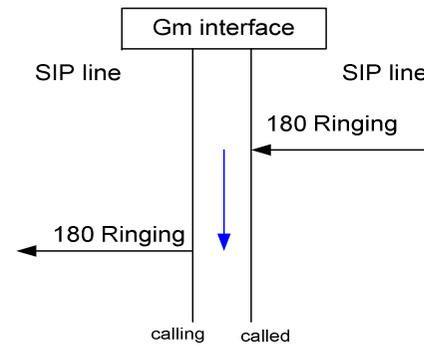
**Figure 7: Alerting sending delay for internal traffic**
