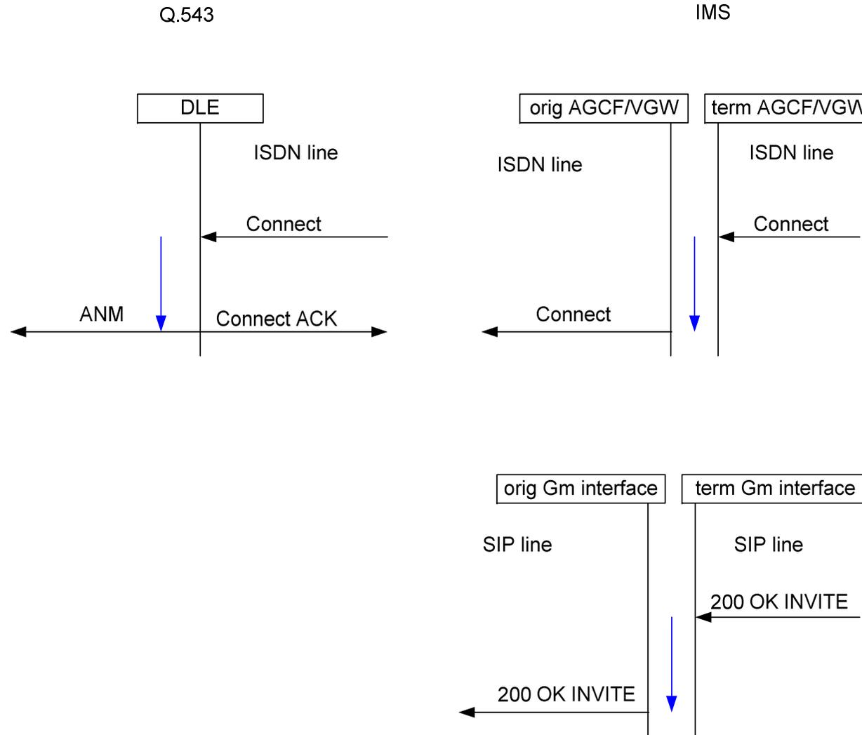
Figure 10: Through-connection delay
