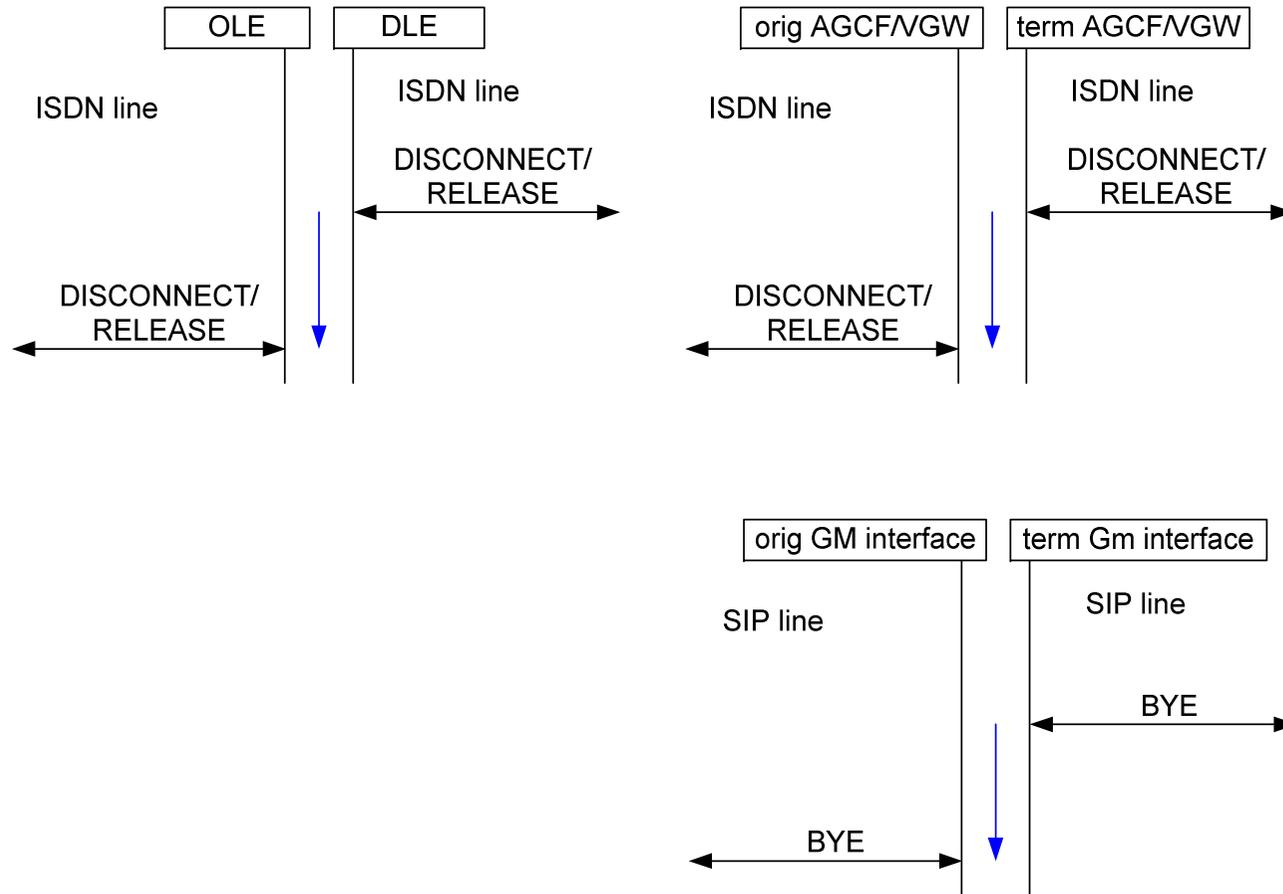
Figure 11: Connection call release delay
