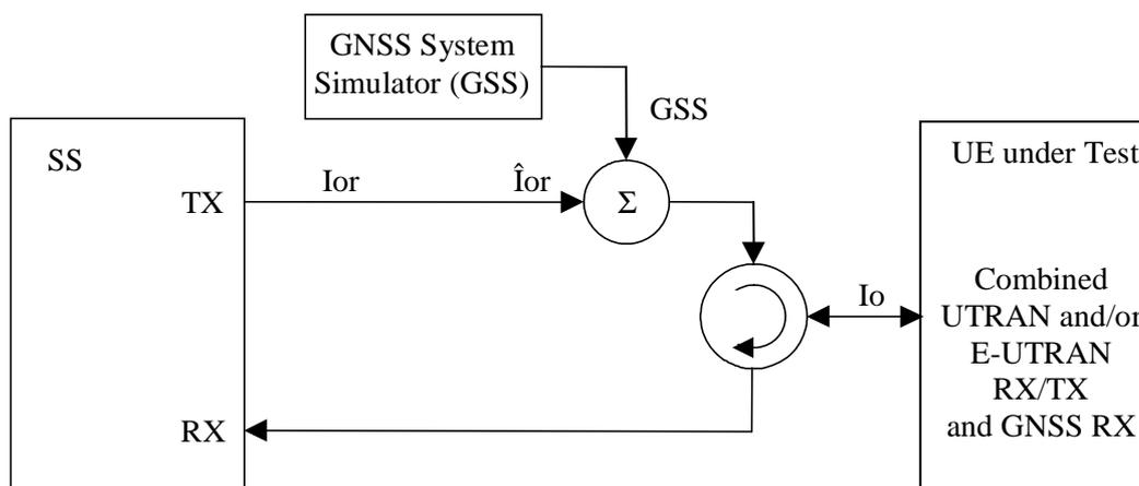
**Figure A.1: Connection for A-GNSS Minimum Performance requirements tests for UE with combined UTRAN and/or E-UTRAN / GNSS antenna**
