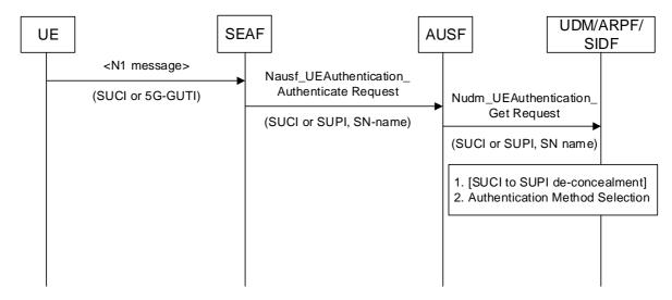
Figure 6.1.2-1: Initiation of authentication procedure and selection of authentication method
