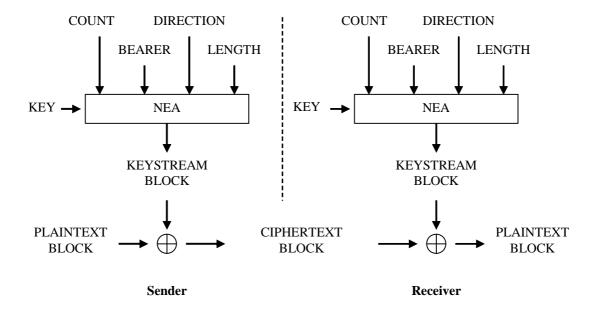
Figure D.2.1.1-1: Ciphering of data
