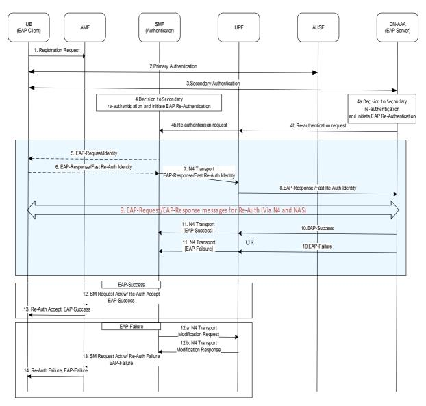
Figure 11.1.3-1: EAP Re-Authentication with an external AAA server
