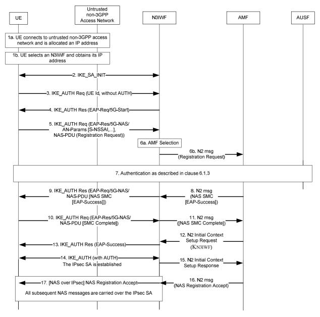
Figure 7.2.1-1: Authentication for untrusted non-3GPP access
