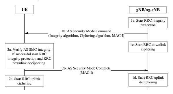
Figure 6.7.4-1: AS Security Mode Command Procedure
