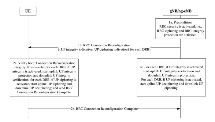
Figure 6.6.2-1: User plane (UP) security activation mechanism
