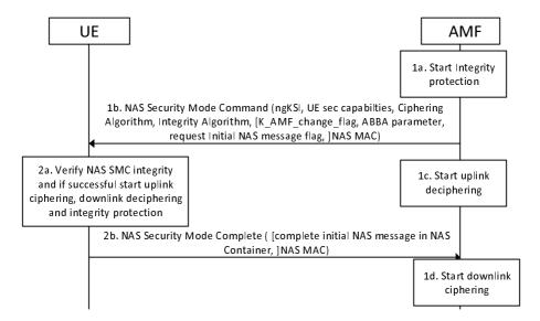
Figure 6.7.2-1: NAS Security Mode Command procedure
