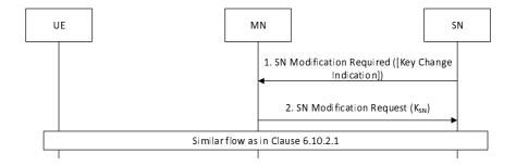
Figure 6.10.2.2.3-1. SN Key update procedure using SN Modification procedure (SN initiated with MN involvement)
