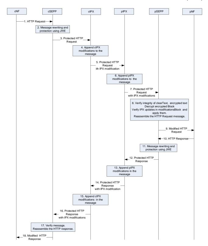
Figure 13.2.4.8-1 Message flow between two SEPPs
