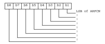
Byte 2: second byte of CPBCCH carrier list element
