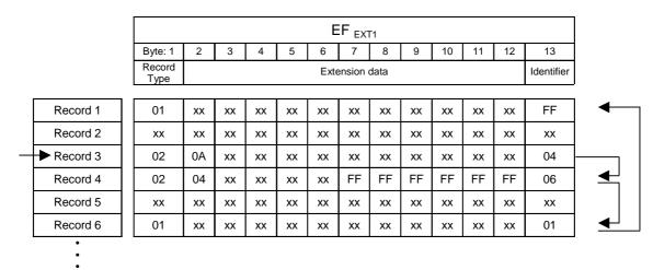
In this example, ADN/SSC is associated to additional data (records 3 and 4) which represent the last 27 or 28 digits of the whole ADN/SSC (the first 20 digits are stored in  $EF_{ADN}$ ) and a called party subaddress whose length is more than 11 bytes (records 6 and 1).
