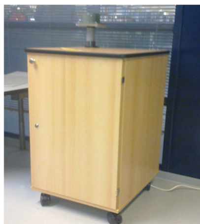
Figure 3: Actual cabinet keeping the SA, omnidirectional antenna and control PC
