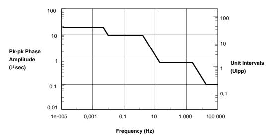
Figure 7: 2 048 kbit/s input jitter and wander tolerance limits
