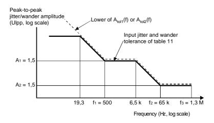
Figure D.3: Upper bound on sinusoidal output jitter at an STM-1 interface [lower of  $A_{tol2}(f)$  or  $A_{tol2}(f)$ ] compared with input jitter and wander tolerance mask
