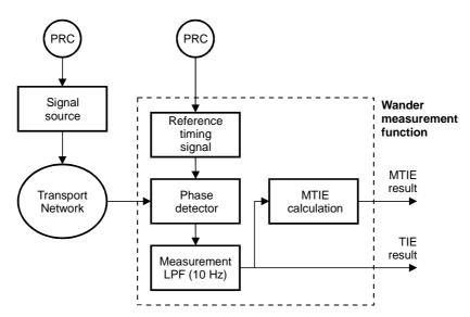
Figure B.1: MTIE measurement of synchronous signals
