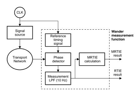
Figure B.3: MRTIE measurement of asynchronous signals, source reference clock available
