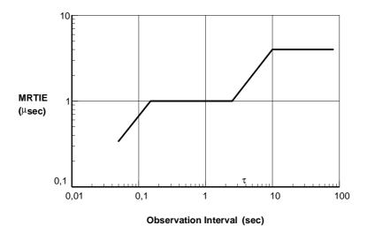
Figure 5: 139 264 kbit/s interface output wander limit
