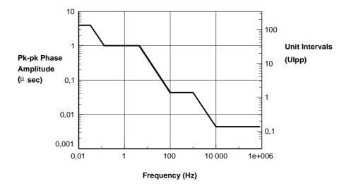
Figure 9: 34 368 kbit/s input jitter and wander tolerance limit
