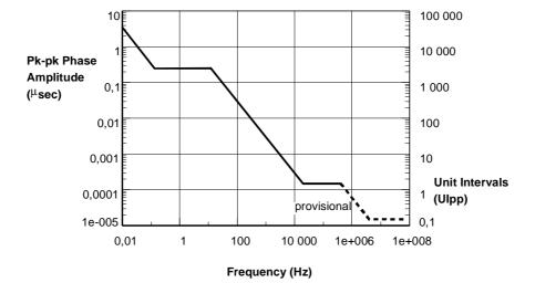
Figure 14: STM-64 input jitter and wander tolerance limit
