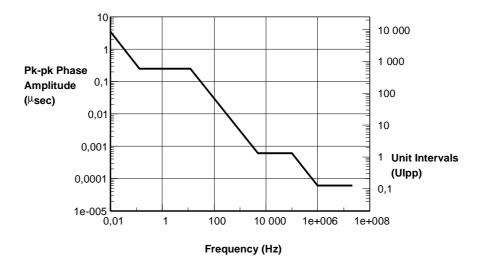
Figure 13: STM-16 input jitter and wander tolerance limit
