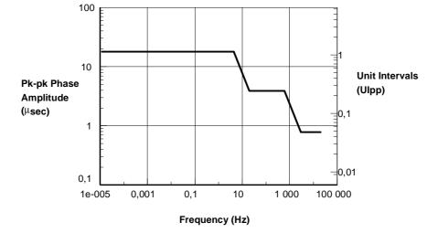
Figure 6: 64 kbit/s input jitter and wander tolerance limit
