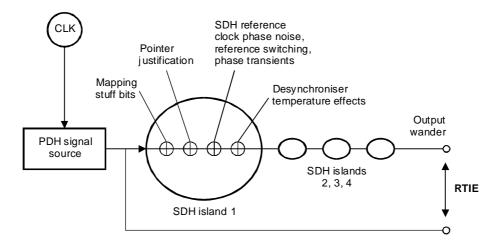
NOTE: CLK frequency offset conforms to bit-rate specifications of ITU-T Recommendation G.703 [15].
