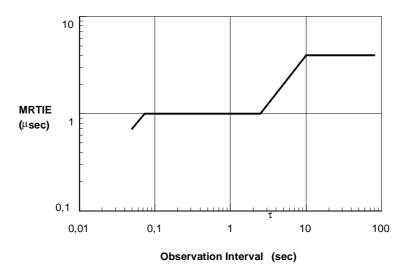
Figure 4: 34 368 kbit/s interface output wander limit
