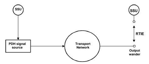
NOTE 1: SSU outputs conform to EN 300 462-3-1 [7] network wander limit. NOTE 2: Both SSUs are traceable to a PRC (but not necessarily the same PRC).
