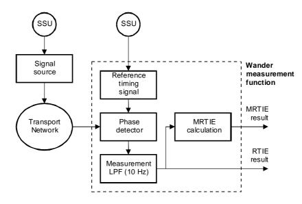
NOTE 1: SSU outputs conform to EN 300 462-3-1 [7] network wander limit. NOTE 2: Both SSUs are traceable to a PRC (but not necessarily the same PRC).
