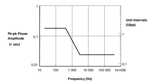
Figure 8: 8 448 kbit/s input jitter and wander tolerance limit
