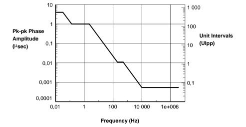
Figure 10: 139 264 kbit/s input jitter and wander tolerance limit
