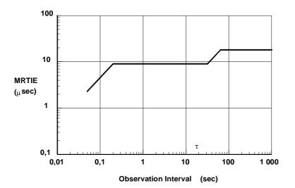
Figure 3: 2 048 kbit/s interface output wander limit
