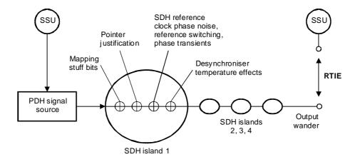
NOTE 1: SSU outputs conform to EN 300 462-3-1 [7] network wander limit. NOTE 2: Both SSUs are traceable to a PRC (but not necessarily the same PRC).
