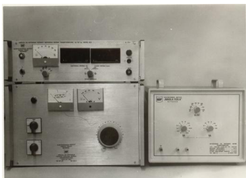
Fig. 10 System for voltage transformers accuracy testing, type NIT-2p (1981.)
