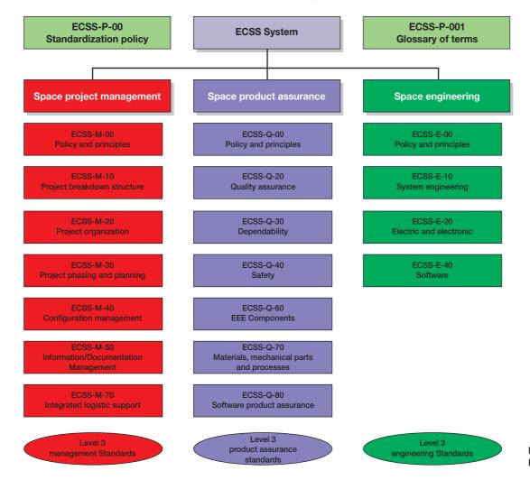
Figure 1. Structure of the ECSS standards
