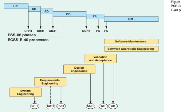
Figure 6. Mapping of the PSS-05 phases to the ECSS E-40 processes
