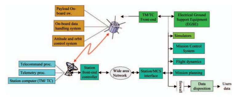
Figure 2. Schematic of a typical space system, with the emphasis on software elements
