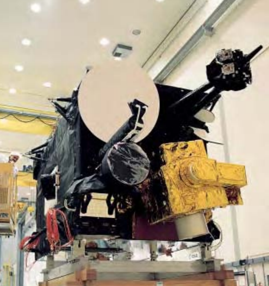
Above: unpacking the Flight Model after its arrival at ESTEC to begin systems-level testing in July 1998. The SILEX terminal is at bottom right; the telescope is pointing down. Above it is the Ku-band feeder link for the LLM land mobile package. At top left is the Ka-band feeder for the SKDR and SILEX packages. Bottom left is the L-band horn for the EGNOS navigation package.
