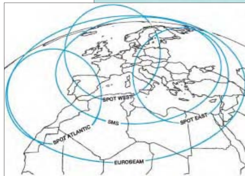
ECS-1 provided services to Europe and north Africa via three spot beams and a single Eurobeam. Its successors added the Satellite Multiservice System for business users.
