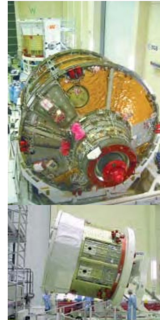
Right/top: the Integrated Cargo Carrier of ATV-1 'Jules Verne' in the ESTEC Test Centre, September 2004. The red covers protect the Russian docking system. The Videometers can be seen in the 8 & 10 o'clock positions. Right/bottom: the spacecraft section ready for mating with the cargo carrier. Below: the ATV Structural & Thermal Model in ESTEC's acoustic test chamber.
