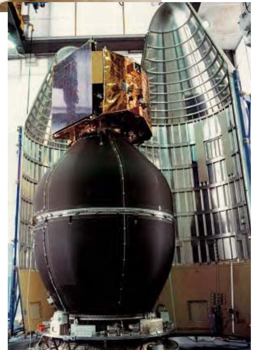
ECS-1 ready for launch. The black Sylda canister carried a second satellite. (CSG/Arianespace)
