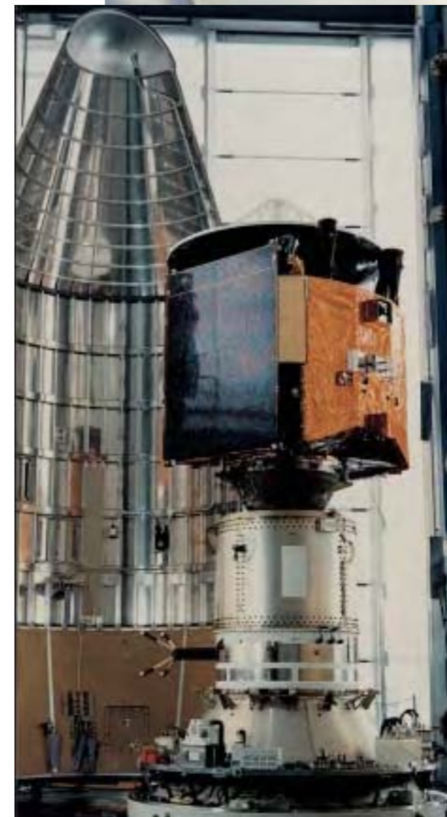
Satellite configuration: maritime version of ECS satellite, 2.2x3.1x1.8 m at launch, solar array deployed span 13.8 m.
