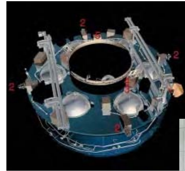
The five Wave Experiment Consortium instruments on Cluster-II. 1: Spatio-Temporal Analysis of Field Fluctuations (STAFF). 2: Electrical Field & Wave (EFW). 3: Digital Wave Processing (DWP). 4: Waves of High Frequency and Sounder for Probing of Density by Relaxation (WHISPER). 5: Wideband Data (WBD). (ESA/VisuLab)
