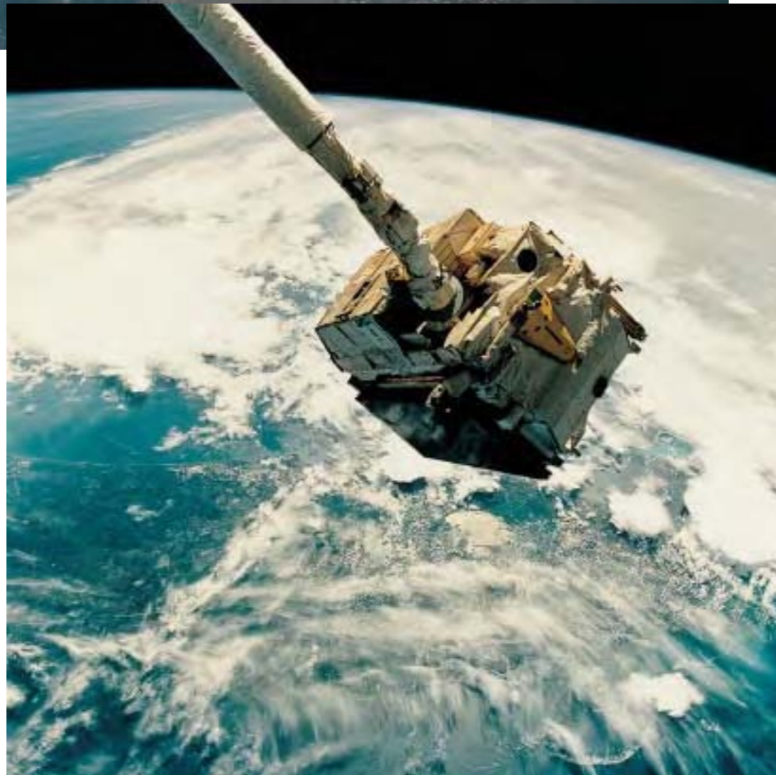
Eureka – with its solar wings already folded against its sides – was recaptured in June 1993 after almost a year in orbit. ESA cost-at-completion for the project was €296.3 million (1983 conditions). (NASA)
