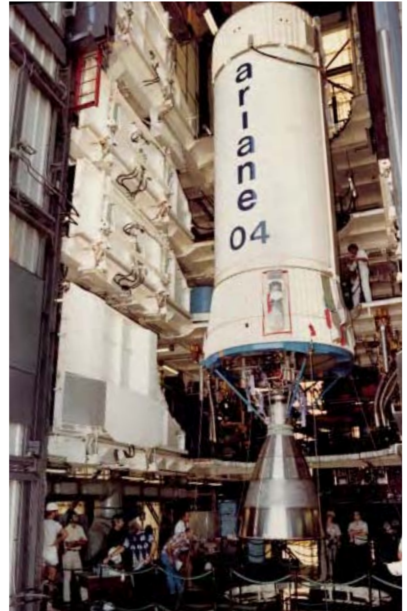
Stage-2 was powered by a single Viking engine. (ESA/CNES/CSG)
