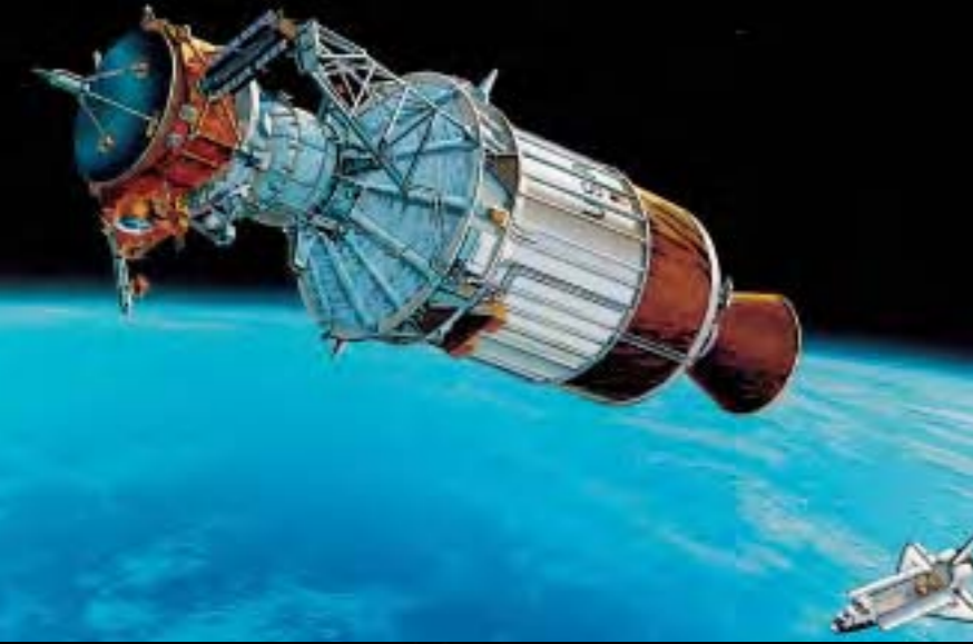
Ulysses was launched on an IUS topped by a PAM final kick stage. (Boeing)
