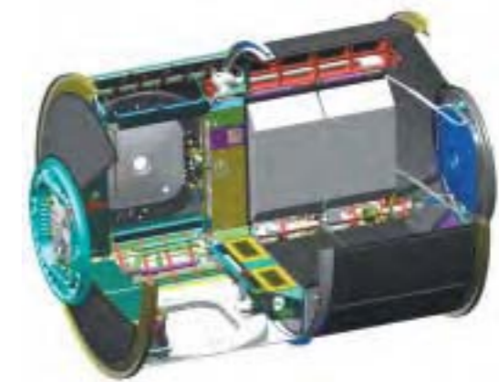
Node-3 internal configuration. (Alenia Spazio)
