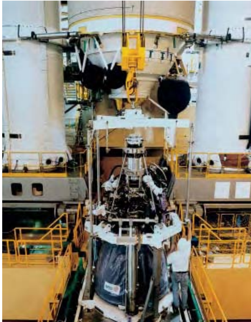
Preparing to install the Vulcain-1 main engine on Ariane-5. (ESA/CNES/CSG)
