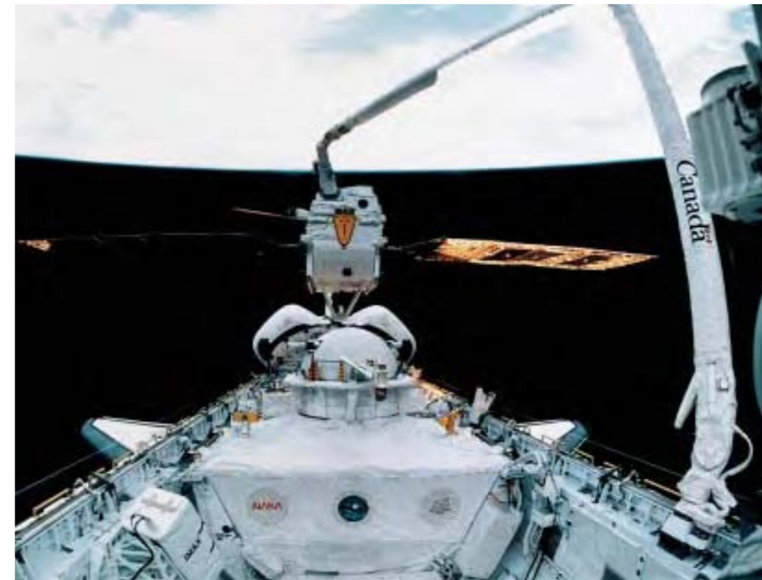
Eureca's solar wings were safely deployed before the free-flyer was released. (NASA)
