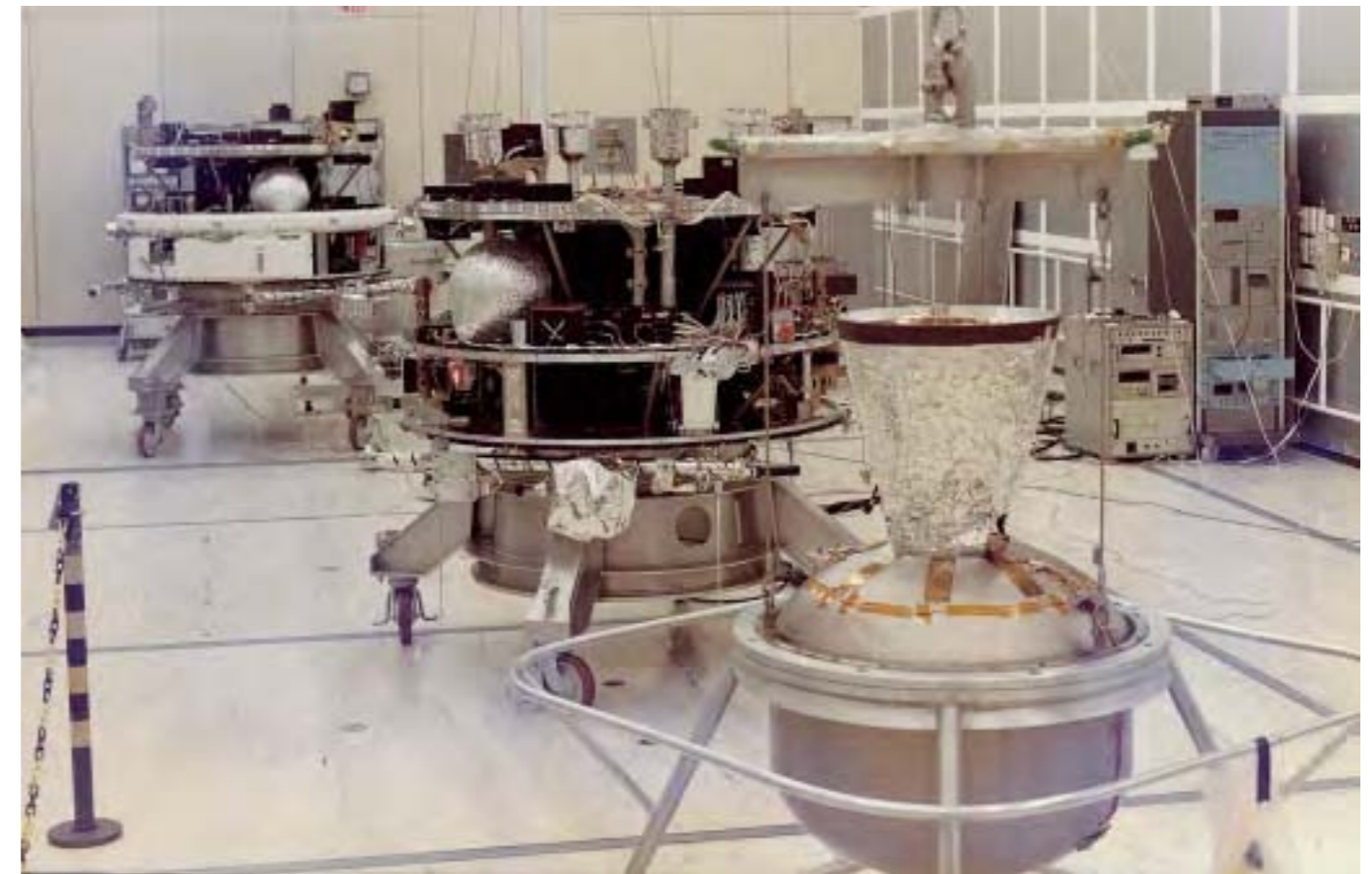
Geos in the Integration Hall at ESTEC. In front of Geos-1 is the Apogee Boost Motor. In the background is the Geos Qualification Model, later modified as Geos-2.
