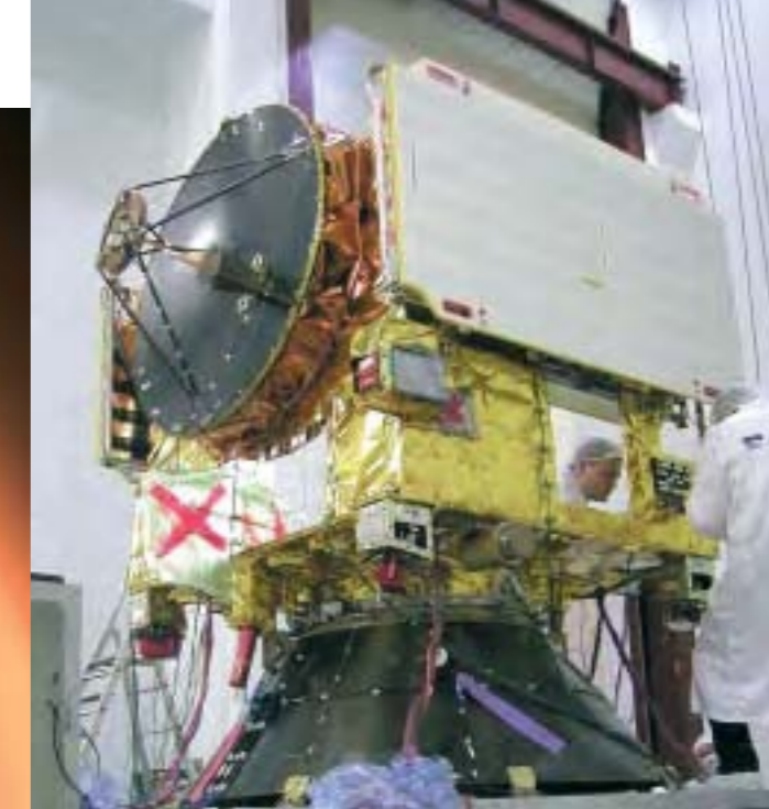
The Venus Express flight model being prepared for vibration at Intespace.
