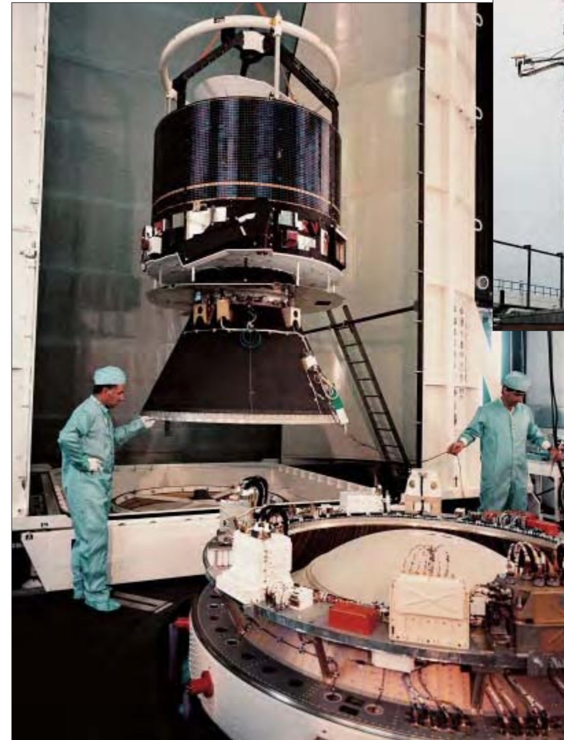
Installation of Giotto on its Ariane launcher at Kourou. The dome cover of Ariane's third stage liquid hydrogen tank can be seen protruding through the centre of the Vehicle Equipment Bay. (CSG/CNES/Arianespace)
