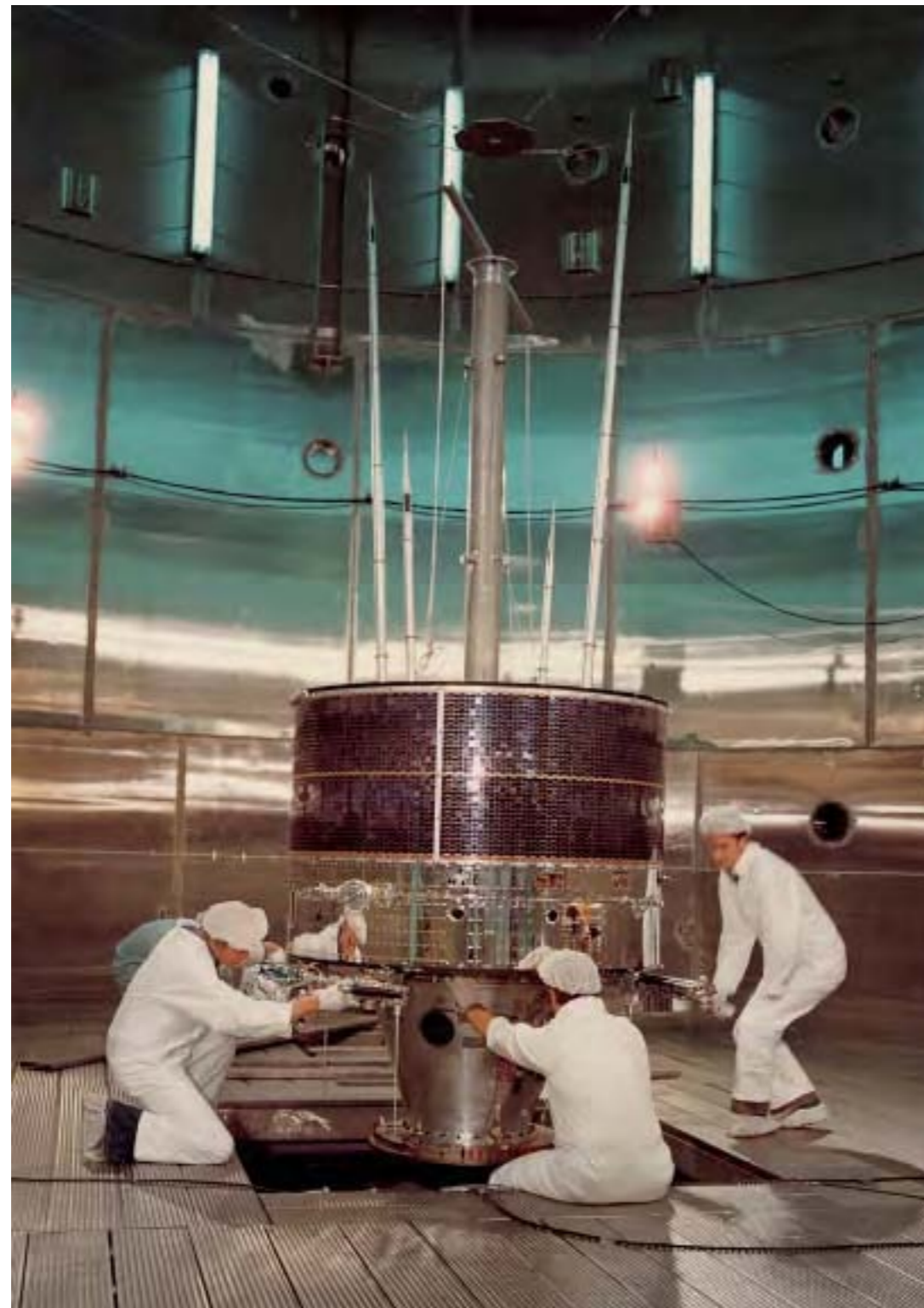
Geos-1 being prepared for boom deployment tests in the Dynamic Test Chamber at ESTEC.
