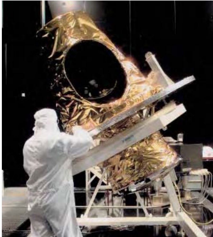
Integration of the SEVIRI Engineering Model at Astrium SAS. The telescope stands 1.3 m high, plus the 1.2 m-high passive cooler for the infrared detectors.
