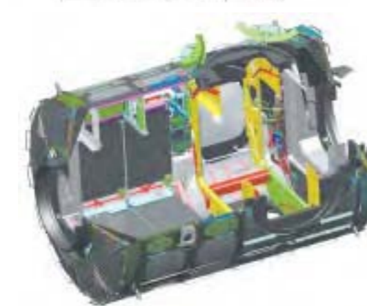
Node-2 internal configuration. (Alenia Spazio)
