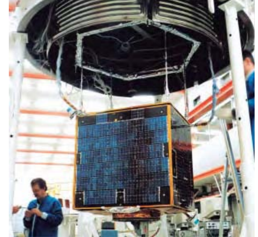
Above: completion of Sloshtsat. The 'spots' on the tank are some of the 270 platinum capacitors for measuring the thickness of water on the wall. Right: Sloshtsat being prepared for thermal-vacuum testing.
