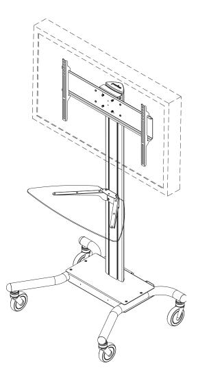
Max UL Load Capacity: 150 lb (68 kg) screen 50 lb (22.7 kg) per shelf
