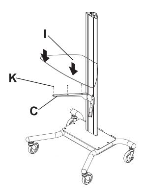
Insert three button bumpers (K) into bottom of shelf clamp bracket (D).
