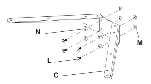
Slide shelf support (**C**) onto upright (**H**) so that 1/4-20 nuts (**M**) slide into slots of upright (**H**) as shown in figure 6 and detail 1. Slide shelf support to desired position, level, then tighten  $1/4-20 \times 12$  mm screws (**L**) using 4 mm allen wrench (**Q**).
