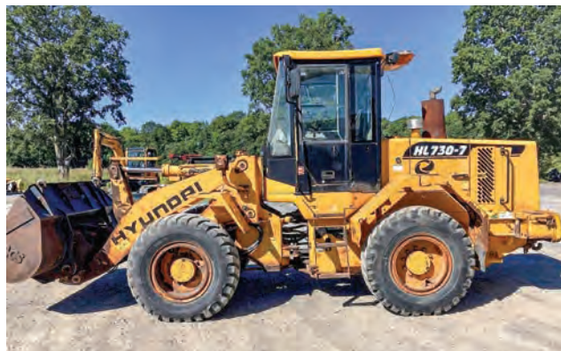
2004 HYUNDAI HL730-7 21384 lb. operating weight, Cummins B3.9C 4 cylinder engine, 125 gross engine horsepower, 4 forward x 3 reverse speed Full Automatic Powershift transmission, 17.5-25 tires, Front & rear fenders, 3rd function auxiliary boom hydraulics, ACS hydraulic coupler, ACS 2 yard material bucket with bolt-on cutting edge ..... $64,900
