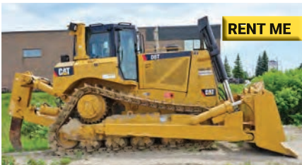
2012 CAT D8T, Cat C15 Acert diesel, Accu-grade ready, good U/C, 4 BBL single shank ripper, semi U blade w/tilt, stk# B130-102
