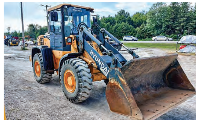
2012 HYUNDAI HL730TM-9 Wheel loader, 26370 lb. operating weight, Cummins 128 horsepower engine, 4-speed Powershift trans., Tool Carrier model with quick-attach, 3rd function aux. hydraulics, 17.5-25 tires, Front & rear fenders, 2.2 yard material bucket with bolt-on cutting edge, Exterior mirrors, Beacon light, Backup camera, 2806 hours ..... $102,900
