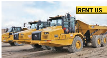
2021 CAT 725 & 730, Cat C9.3/C13 Acert diesel 320/375 hp, 26.5/31 ton payload, drive, stk# B145-180/B145-179
