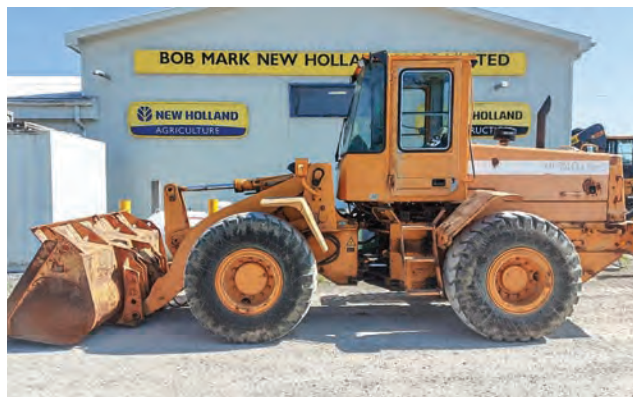
1999 HYUNDAI HL740XTD-3 Wheel loader, Extended reach/High lift model, 25350 lb. operating weight, Cummins QSB5.9 engine with 140 hp, Bateman 3.0 cubic yard Q/A bucket with bolt-on cutting edge, Bateman Hyd. QC, 20.5-25 tires, Front & rear fenders, 4 forward x 3 reverse speed Powershift trans, Aux boom hyd. 4233 hours ..... $44,900
