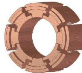
Fig. 2 Three dimensional schematic view of the segmented ring electrode
