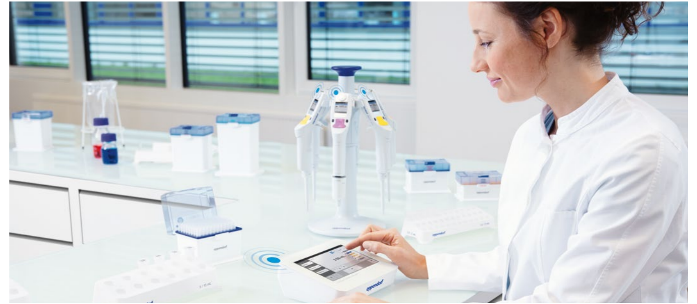
VisioNize pipette manager External touch server to enable communication with connected electronic pipettes as standalone systems
