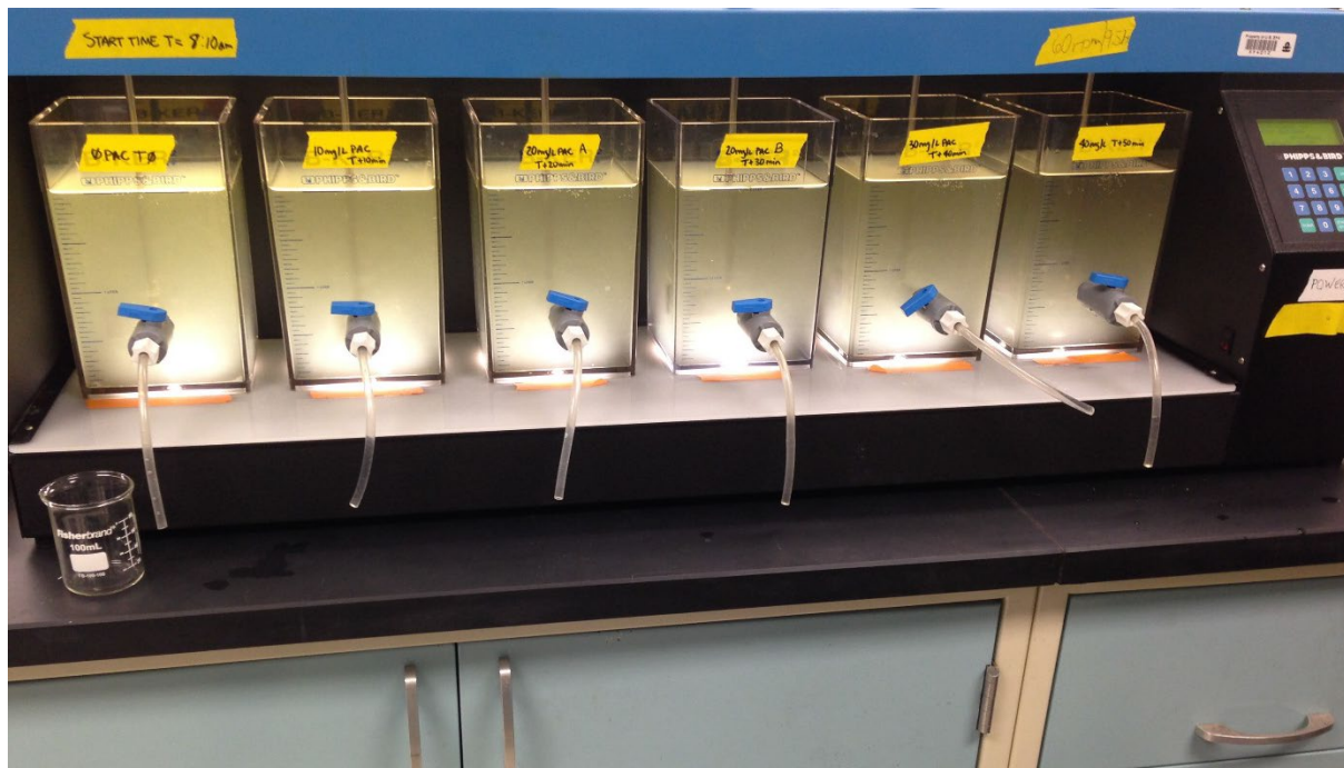
FIGURE 24. Jar testing to simulate impact of variable PAC dosages and contact times on microcystins concentrations.
