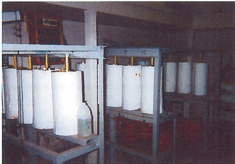
Figure 1. Incubation schematic and photograph of multiple cells maintained at various constant temperatures.
