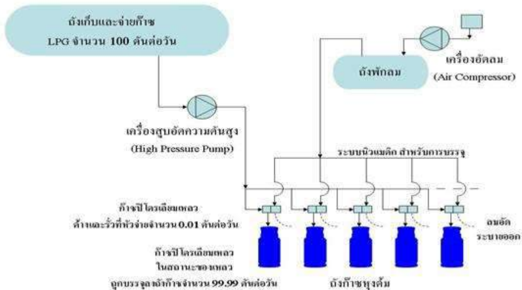
Gas cylinder filling system
