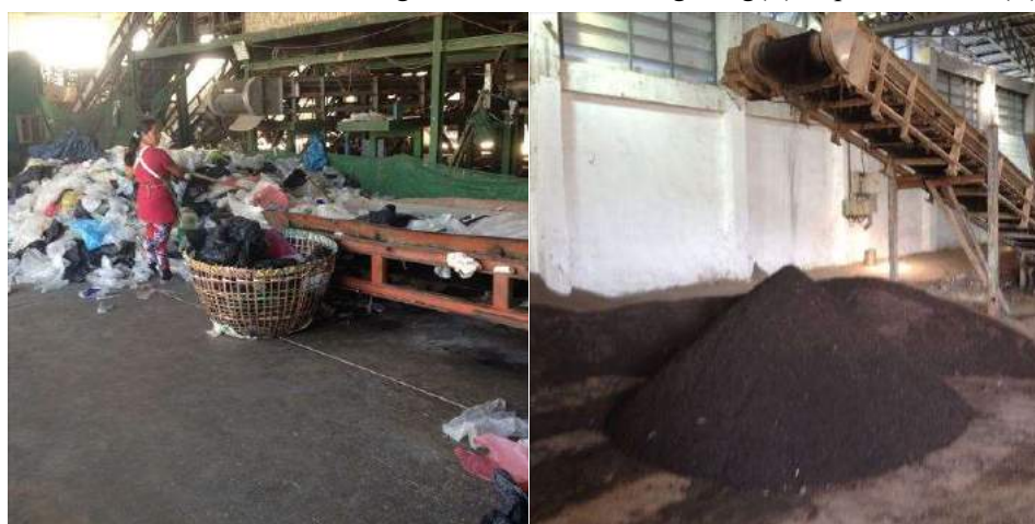
Second Sorting of Plastic Waste(L) & Compositng Line (Final Process) (R)
