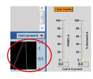
In this example, the evc/epc declared an error because the output current 1.16A is **0.5A higher** than the max setting 0.63A.
