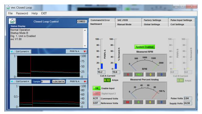
The closed loop control is a dynamic process. The evc/epc constantly changes the current to maintain the reference rpm.
