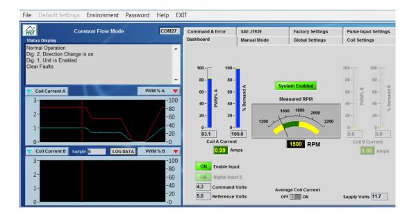
Constant Flow Mode operates with a variable displacement pump.
