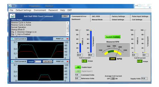
The Anti-Stall function reduces the current to prevent the engine from stalling during a sudden external load increase. The fixed set-point determines the max forward speed of the work function. The reverse set-point determines the max reverse speed of the work function.
