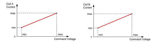
**Coil Selection Active** (Enabled/OFF) – when **enabled**, Analog Center Active is automatically turned **OFF**. 0-5V gives both coils 0-100% PWM current output. But there is only one output at one time.
