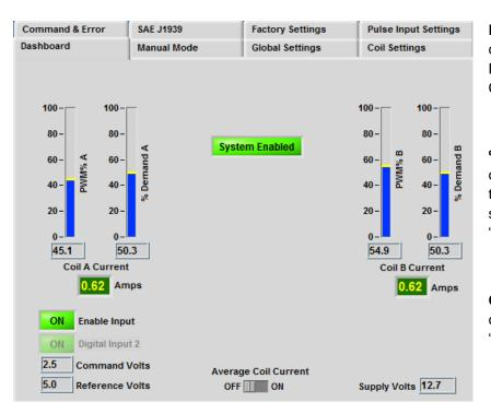
**PWM% A/B** – displays the PWM duty cycle output for coil A and B. The PWM% B will be "Grayed Out" when Coil B is disabled.
