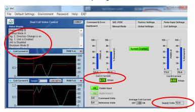
They give real time overview of the controller health, operation of the system and condition of inputs, outputs and any alarms.
