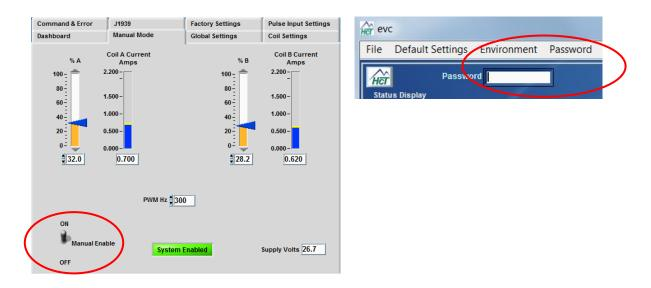
"Manual Mode" provides a quick method of testing the outputs. Manually verify that the system is working properly and determine the max coil current for the present operating conditions.
