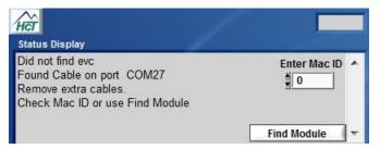
The **MAC ID** determines the module's Command and Status PGN addresses on the SAE J1939 bus. The user may command multiple evc/epc modules on a single SAE J1939 bus. Please see SAE J1939 section.
