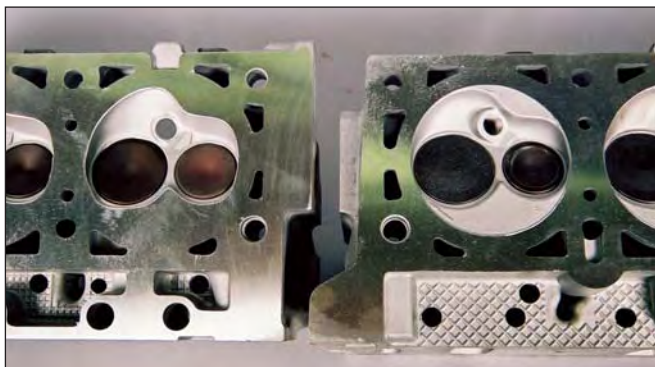
Chrysler modified the chambers and relocated the spark plugs for the '01 heads (right).
