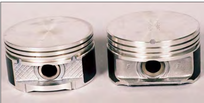
The piston for the 3.8L (left) is smaller in diameter and has a lower compression height than the one for the 3.3L (right).
