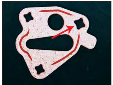
The gasket for the oil filter adapter had two 8.0mm holes and one 10mm hole (with arrow) in '07-'10 instead of the three 8.0mm holes that were used for the '01-'06 applications.
