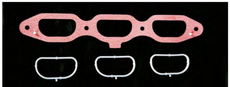
The aluminum intakes used two of the fiber gaskets (top) instead of the individual molded ones (bottom) that were used for the plastic intakes.
