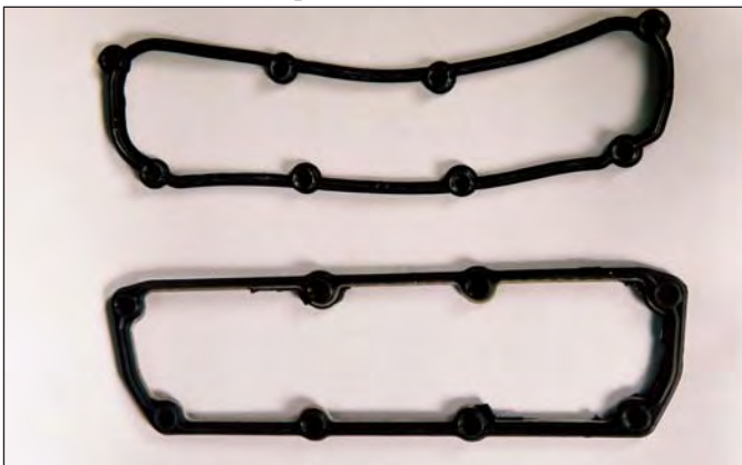
The rigid rocker gaskets for the stamped steel covers are on the bottom and the flexible ones for the plastic covers are on the top.
