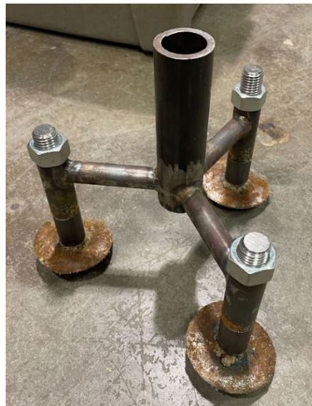
Figure 11: Fully assembled foundation, with augers, stops, and hex nuts attached.
