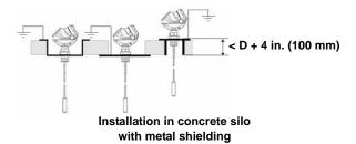
To prevent an extremely high tensile load when fixing the probe, and to reduce the risk of probe breakage, the probe must be slack. Select a probe longer than the required measuring range so that there is a sag in the middle of the probe that is greater than or equal to 1<sup>1</sup>/<sub>2</sub> in. per 10 feet (1 cm per m) of the probe length
