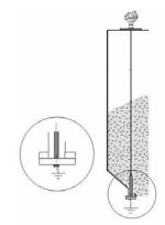
Grounding the probe end in products building up static electricity
