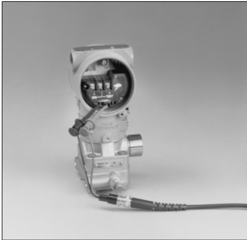
FIGURE 4-2. Connecting a Personal Computer to a Model 3095FT.
