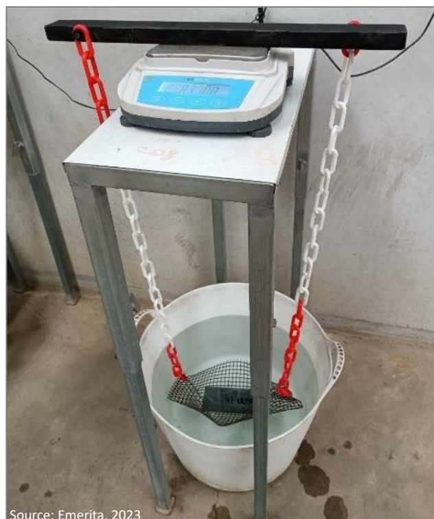
Figure 11.3: U.S. Solid USS-DBS28-30 Balance Taking a Wet Weight for Bulk Density Calculation
