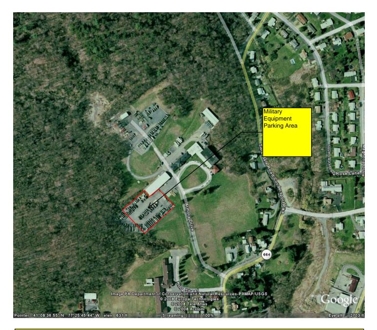
The above referenced Military Equipment Parking Area is approximately 7,200 S.Y. The contractor will be required to design and Construct a repair/replacement project +/- 5,200 S.Y. The area designated in red above (approx. 5,200 S.Y.) shows the area of priority for this pavement project. All fencing will be removed and replaced as part of this project, along with all existing gates.
