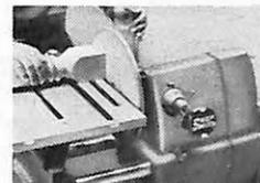
The Mark V as a lathe offers exceptional capacity with a 16½" swing for face-plate turning. Speed Dial allows a speed range of 700 to 5200 rpm.
