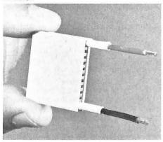
Two of these miniaturized thermoelectric modules replace all the bulky complex piping coils, compressors and motors in conventional portable refrigerators. The modules pump heat from your food into efficient heat sinks where it is dissipated by a quiet fan. They operate on a principal called the "Peltier Effect" - passing electricity through the junction of dissimilar metals causes heat to flow away from the junction
