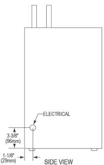
NOTE: When mounting unit in an open area, to ensure proper ventilation, maintain a 4" (102mm) clearance from cabinet louvers on each side of chiller. When mounting unit in a cavity or behind a wall, maintain minimum space of 4" (102mm) on each side, 4" (102mm) on the top and a depth of 12" (305mm).
