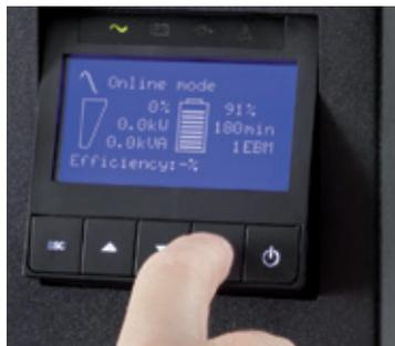
9SX LCD tilts 45° for ease-of-viewing
