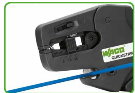
Cutting a conductor.
