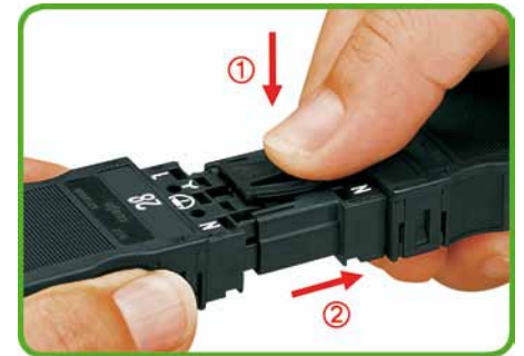
Locking lever, manually operated: 1.) Press on locking lever. 2.) Pull apart the connectors.
