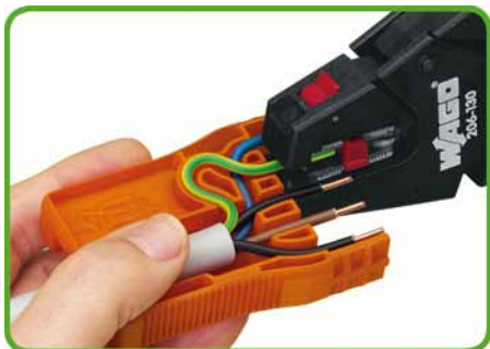
Strip conductor ends 9 mm (see marking).
