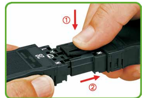
Locking lever, manually operated: 1.) Press on locking lever. 2.) Pull apart the connectors. (Example shows 3-pole connectors)
