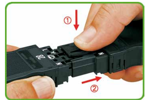
Locking lever, manually operated: 1.) Press on locking lever. 2.) Pull apart the connectors. (Example shows 3-pole connectors)
