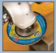
Several different designs offer the user ways to enhance both the performance of the disc and the final results left on the workpiece. Choose from shapes in flat,  $6^{\circ}$  convex shape, or  $12^{\circ}$  convex shape. Flat discs are best suited for use on flat surfaces and on edges. The  $6^{\circ}$  convex shape allows for use on flat or slightly contoured surfaces, while the  $12^{\circ}$  convex shape is perfect for contoured surfaces.
