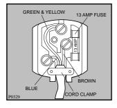
Connect the green and yellow (earth) wire to the terminal in the plug which is marked with the letter «E» or the earth symbol  $\bot$  or coloured green and yellow.
