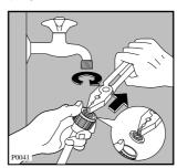
Turn off the water taps. Unscrew the water inlet hoses. Remove and clean the filters using a hard bristle brush. Replace the filters and tighten up the inlet hoses.
