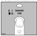
Depress the ON/OFF button: the mains-on light comes on and the machine starts operating.
