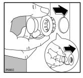
Slide out the 3 plastic spacers and plug the 3 holes with the 3 plastic plugs which are supplied with the instruction booklet.
