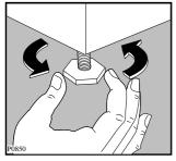
Level the washing machine by raising or lowering the feet. The feet may be tight to adjust as they incorporate a self locking nut, but the machine MUST be level. Any necessary adjustment can be made with a spanner. Accurate levelling
