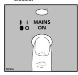
Depress the ON/OFF button: the mains-on light illuminates and the machine starts operating.
