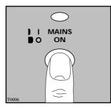
Depress the ON/OFF button, the mains on light and drying light will illuminate and the machine starts operating.
