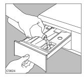
Pour the fabric softener, if required, into the compartment marked \&\mathbb{B}.
