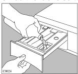
Pour the fabric softener, if required, into the compartment marked & .
