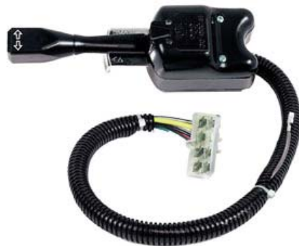
vsm910Y601 Replacement Turn Signal Switch for: Mack 1MR572
