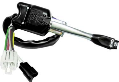
vsm915Y103 Replacement Turn Signal Switch for: KENWORTH K301D230;18500D044 • 8 wire harness • Handle features built-in push button high/low beam selector switch • 16 bulb capacity for hazard warning • 8 bulbs per side for turn signal flashing
