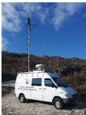
Mobile control-measuring station (MKMS) in the vehicle Mercedes-Benz® Sprinter
