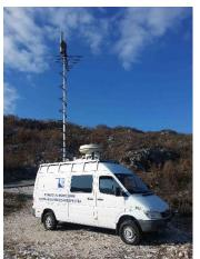
Mobile control-measuring station (MKMS) in the vehicle Mercedes-Benz<sup>®</sup> Sprinter
