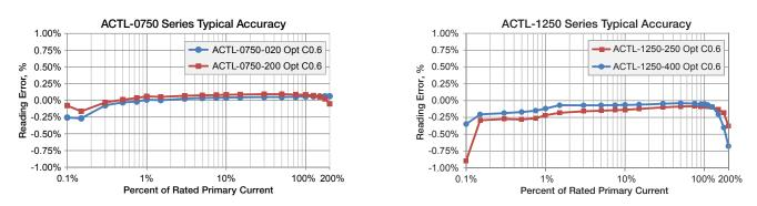
Graphs show typical performance at 23°C, 60 Hz. Graph shows a positive phase angle when the output leads the primary current.
