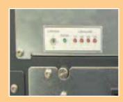
Fan failure display/ four speed levels
