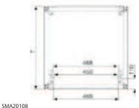
h d Model Order no. UP W Н D U kg 612 12 28 02.110.212.1 600 600 1 unit 36 02.110.222.1 600 879 600 18 1 unit 44 02.110.232.1 600 1146 600 24 1 unit 600 612 800 12 32 02.110.214.1 1 unit 40 02.110.224.1 600 879 800 18 1 unit 02.110.234.1 600 1146 800 24 48 1 unit
