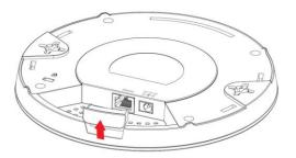
**2.** Connect a router or PoE switch to the access point's LAN port using an Ethernet cable.
