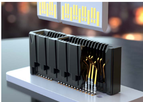
High-Speed Differential Pair Edge Card connector uses Samtec's Edge Rate® contact system to support high-mating cycles and 28 Gbps performance.
